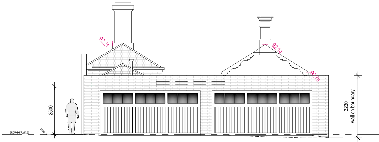
EAST ELEVATION (parapet roof + panelled doors)
