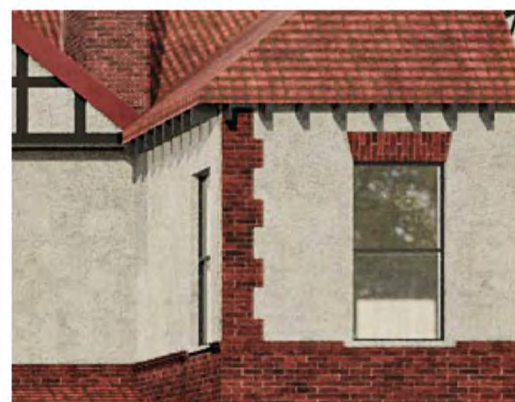
DUMMY RAFTERS PAINT RESENE 'IRONSAND' OR SIMILAR
