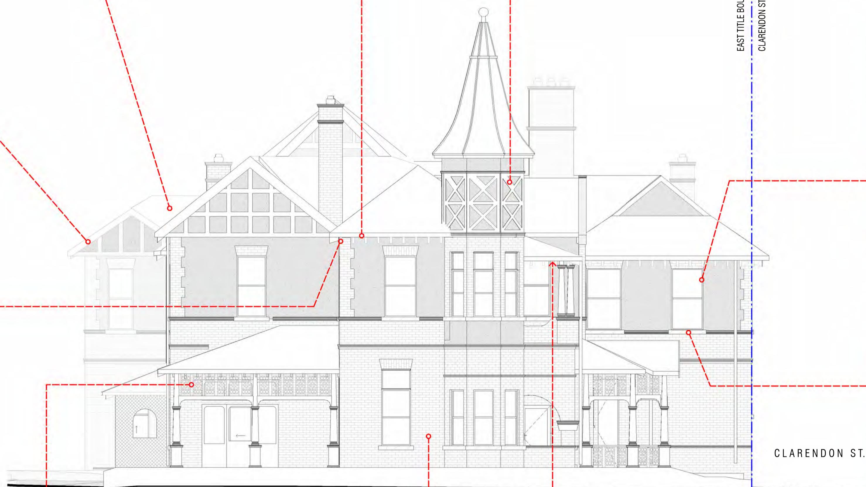
WINDOW FRAMES & GLASS MAKE GOOD EXISTING WINDOW FRAME, TREAT DECAY TIMBER FRAME PAINTED WITH RESENE 'IRONSAND' OR SIMILAR REPAIR MECHANISMS, CORD, WINDOW SEAL TO MAKE WINDOWS OPERABLE AND SMOOTH. REPLACE SINGLE FLOAT GLASS WITH LAMINATED SAFETY GLASS FOR CODE COMPLIANCE
