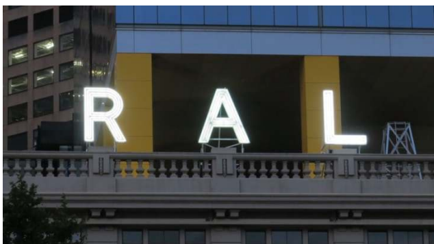
Colour Test illustration: Colour comparison to be made between LED rope and the repaired Neon Tube letter A. It is just apparent that letter R is very close in colour to letter A.
