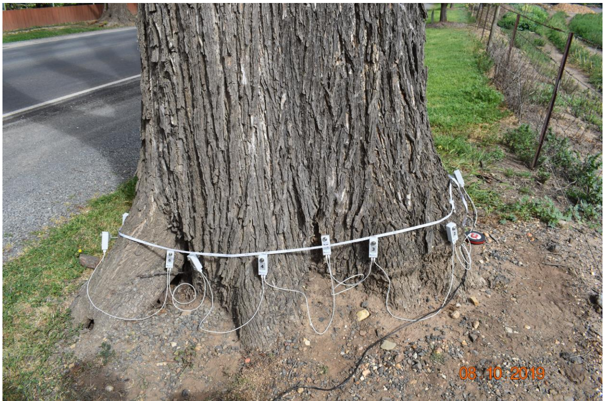
Figure 8: Arbotom® sensors around the subject tree.
