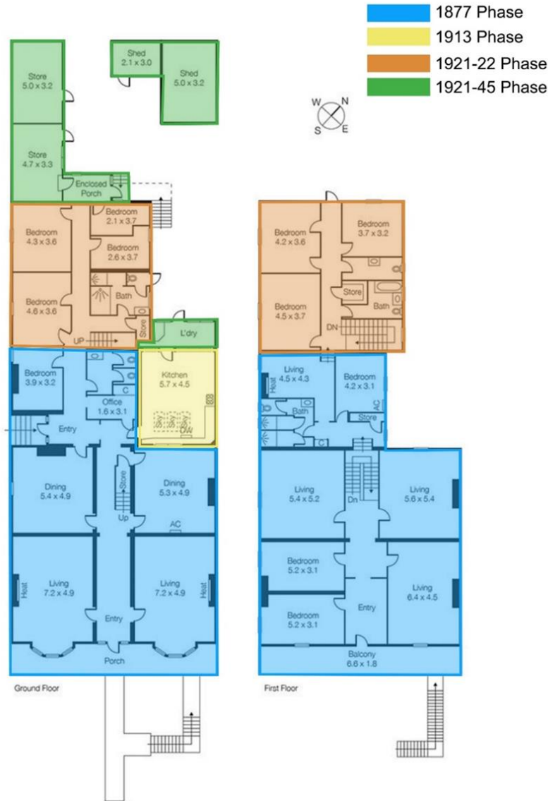
Hambleton House, phases of development (Source: RBA Architects, Hambleton House CMP , 2024 p10)
