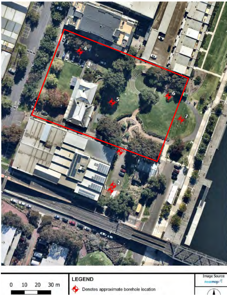
Figure 20 Borehole testing location within the study area (red) (GeoAust Geotechnical Engineers Pty Ltd, 2023)
