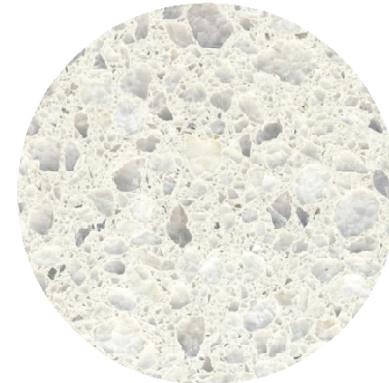
FL08 - OVERPASS FLOOR COLOUR: WHITE CEMENT, WHITE AGGREGATES; WHITE PIGMENT/OXIDE. LOCATION: OVERPASS
