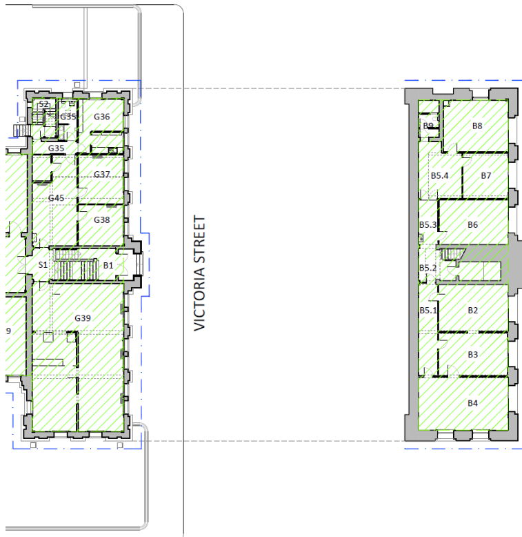
Figure 2 Basement (right) and ground (left) floor plans of Stage 9 (Victoria Street wing) indicating works areas (green shading) included in the project Source: Lovell Chen, Drawing No. A-001, June 2024
