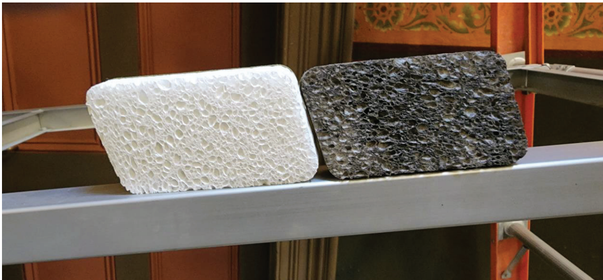
Figure 15 Comparison between clean and soiled sponge on east wall.
