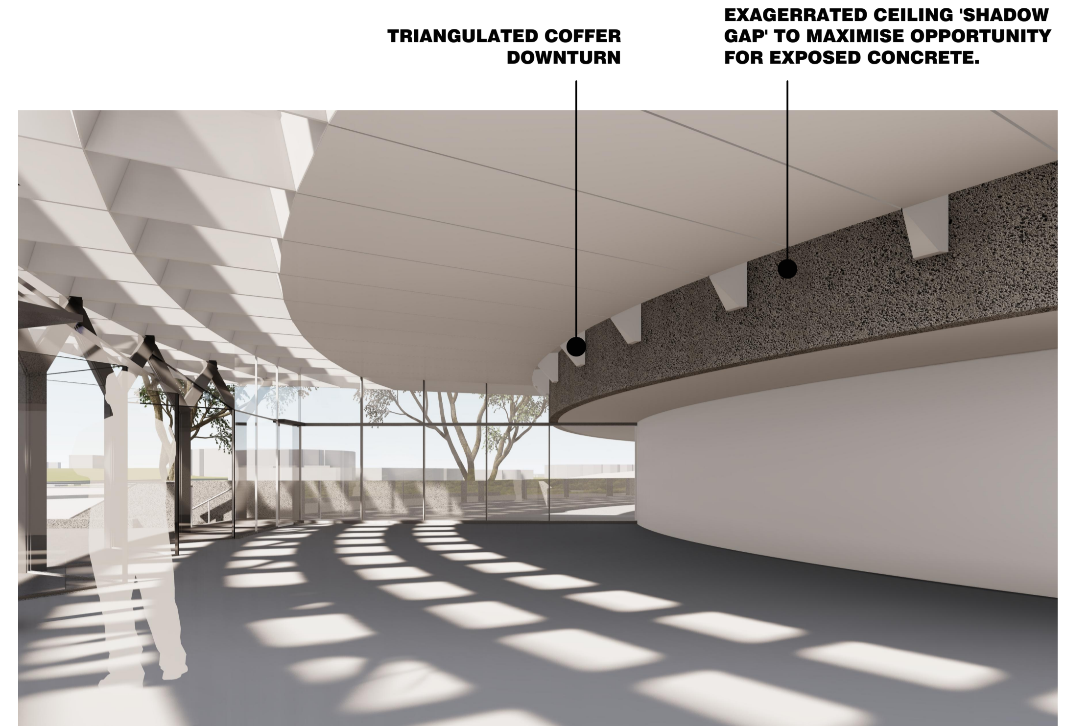
NORTHERN CANOPY CEILING (NOTE : INDICATIVE DESIGN ONLY TO BE CONFIRMED / DELIVERED AS PART OF TENANCY FITOUT)
