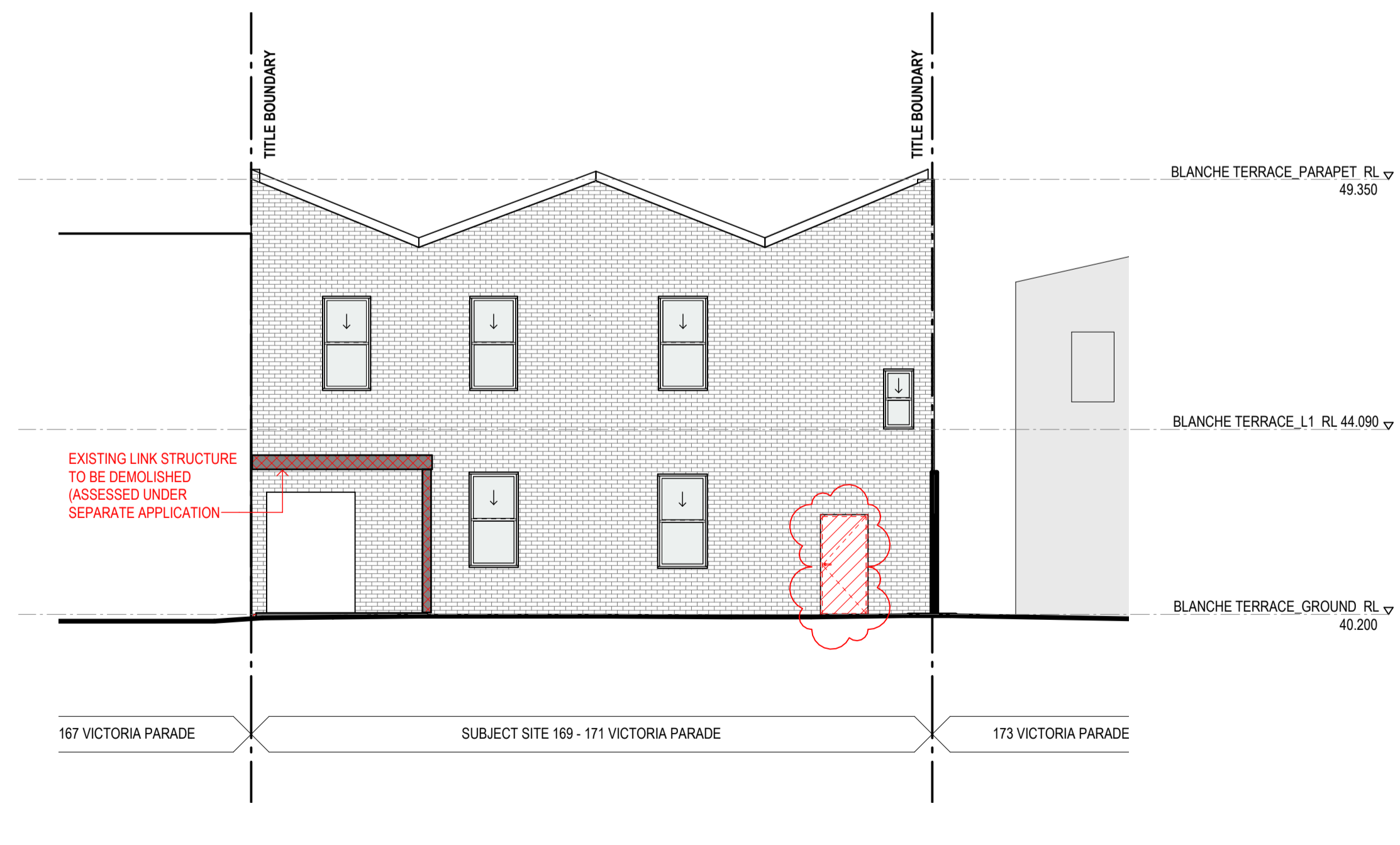
4 DEMOLITION NORTH ELEVATION - VIC PDE (INTERNAL COURTYARD) 1:100
