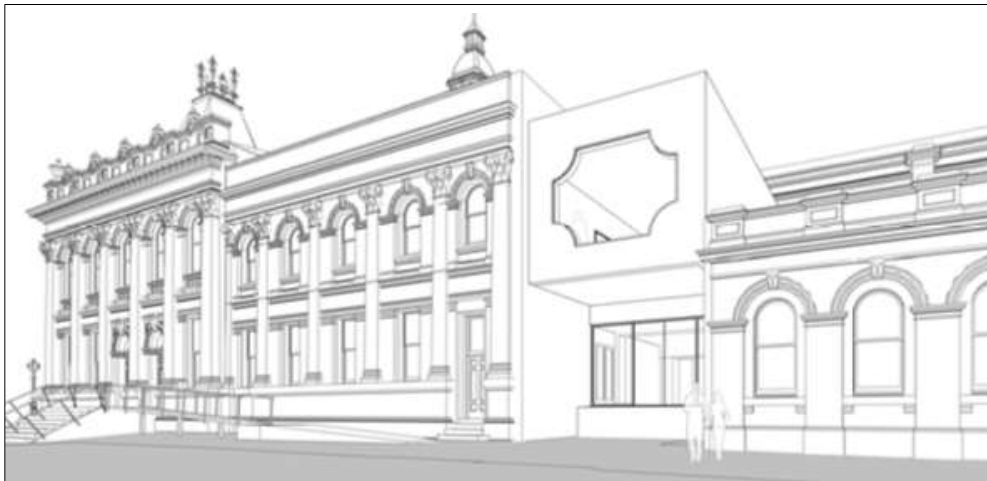
Figure 40 Architect's illustration showing proposed first floor addition built over the existing 1990s loading bay.
