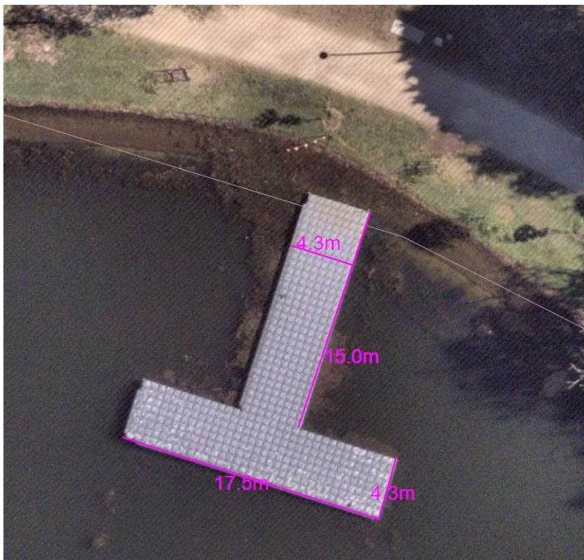
Figure 4: Dimension and configuration of the Pontoon. This may be reconfigured as required, including floating off shore with an additional 17.5 x 4.3m float brick
