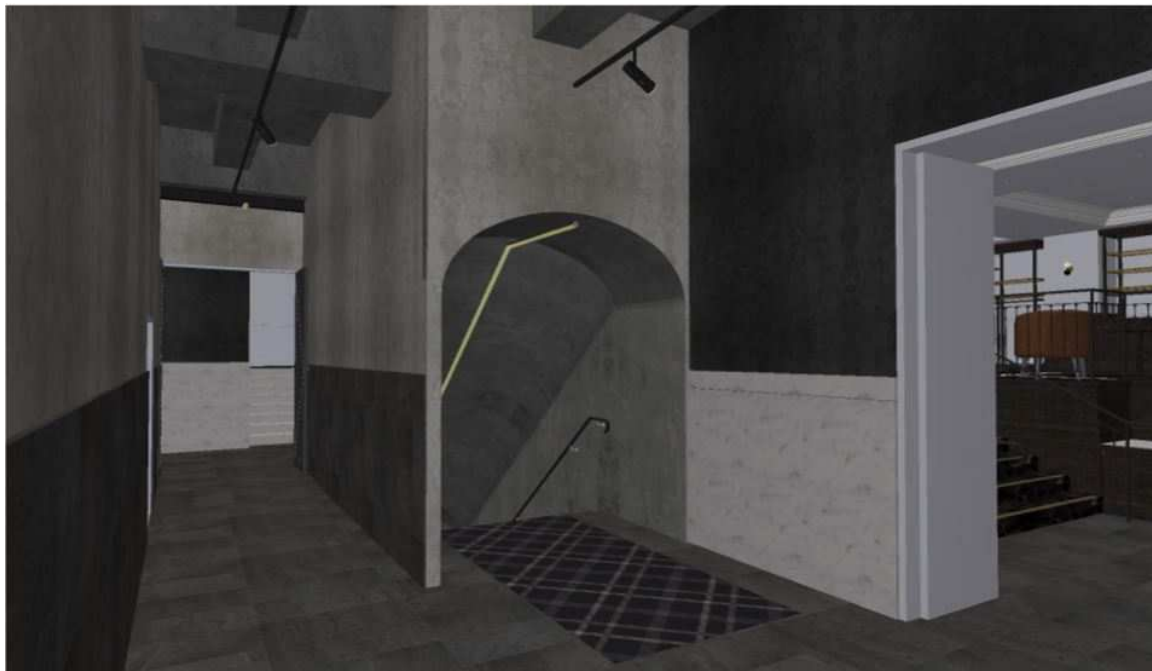
Figure 9: Render view of the lobby area, showing the new vaulted ceiling to the stair. Source: Extract of drawing B210, Studio Y.
